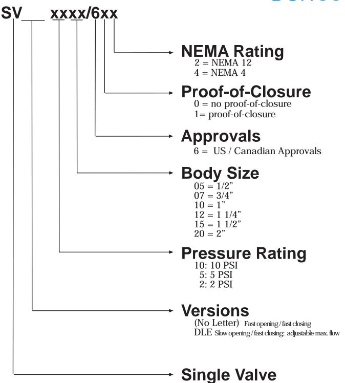
Note: The nomenclature does not indicate an operating voltage. A specific part number must be used to indicate the desired coil voltage
